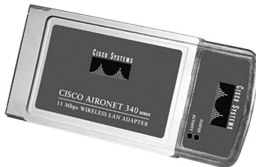
Figure 1.3 A wireless LAN adapter for a notebook computer from Cisco Systems.
