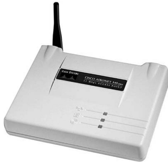
Figure 1.2 A wireless LAN access point, the Cisco Aeronet 340.
